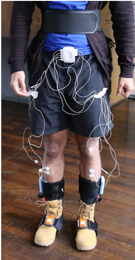
Figure 1: Experimental setup – Xsens and PLUX sensors are applied.
